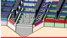
Internally contoured profiles allowing for the inclusion of separate heating zones within the furnace, ensuring optimum temperature profile.
